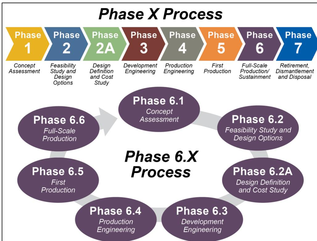
**Figure 2–4. Phase X and the Phase 6.X Process**
