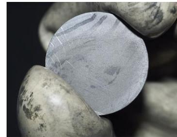
*A small disk of plutonium metal at TA-55.*
