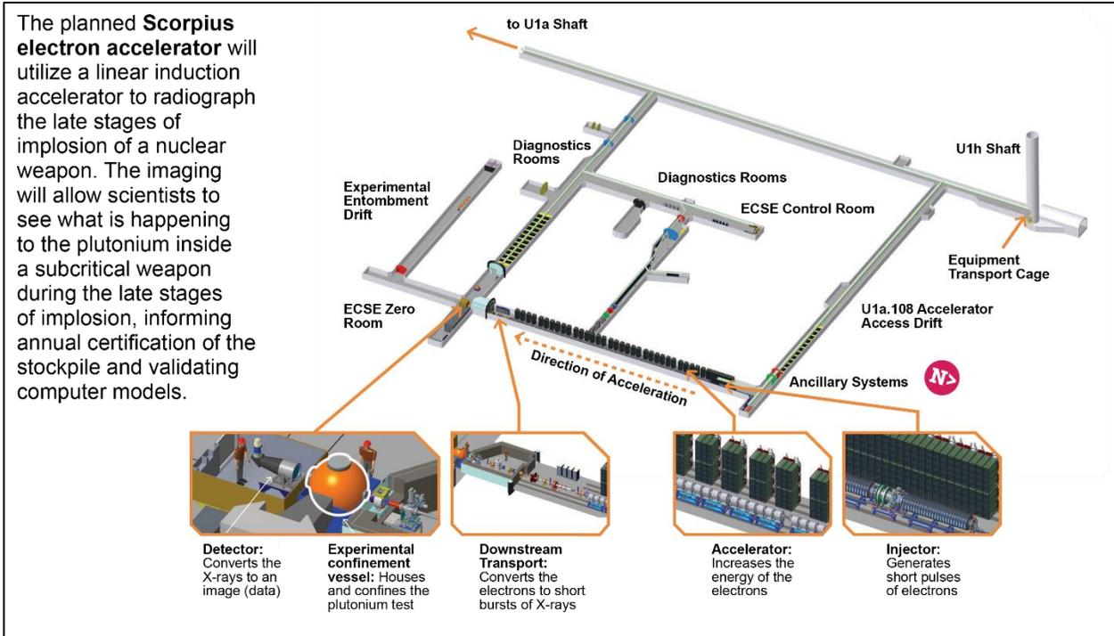
**Figure 4–5. Advanced Sources and Detectors “Scorpius” Layout at U1a Complex**
