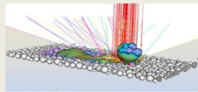
**A laser interacting simultaneously with the melt pool and a large “spatter” of metal powder particles**
