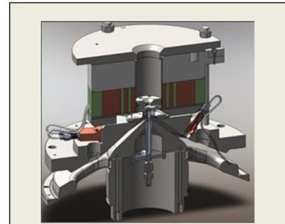
**Cutaway Diagram – Z Beamlet Transport Tube**
