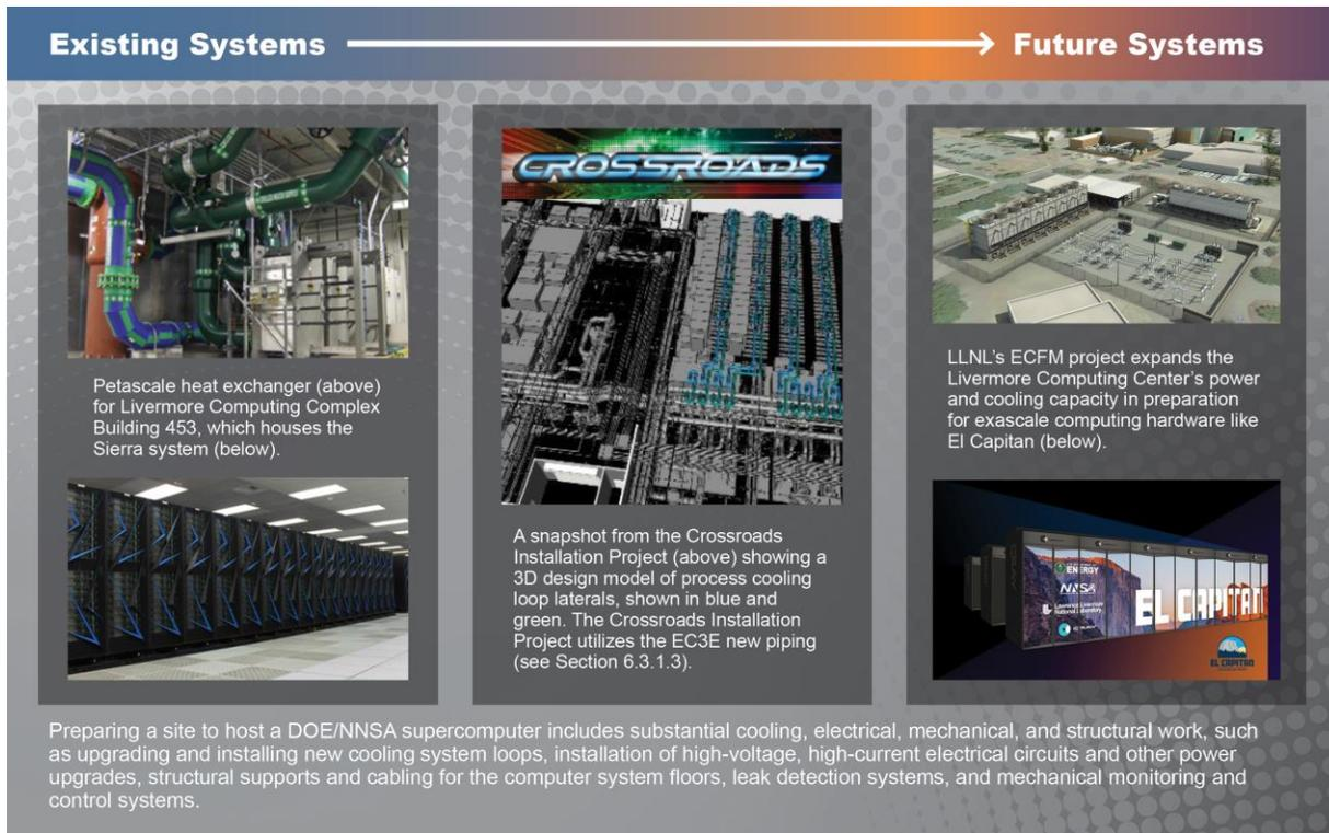
**Figure 6–4. Integrated mission and infrastructure planning is crucial to the success of DOE/NNSA missions, as illustrated by this example from Weapons Simulation and Computing**
