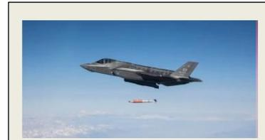
*An F-35A opens its bomb bay doors and drops a mock B61-12 at Sandia National Laboratories' Tonopah Test Range. It was the first of a testing series that will conclude with full-weapon systems demonstrations designed to increase confidence the bomb will always work when needed and never under any other circumstances.*
